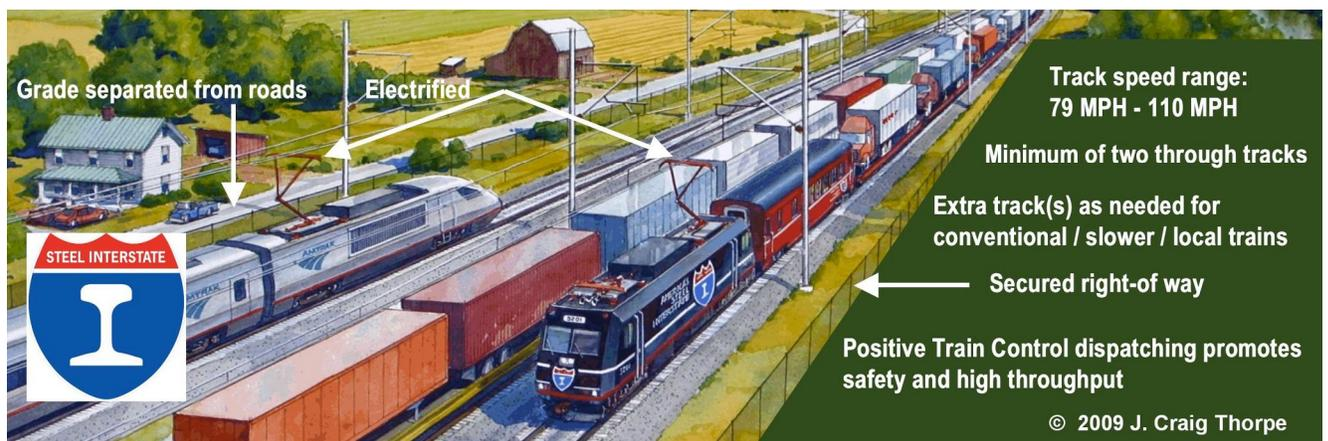
***ELEMENTS OF STEEL INTERSTATE DESIGN:*** A minimum of two grade-separated *through* tracks, engineered, signaled, and dispatched for 79 MPH to 110 MPH, offering frequent, reliable service. The electrified Steel Interstate System would create adequate capacity to divert most non-local truck freight to intermodal trains, and to accommodate passenger trains without impairing freight operations.
