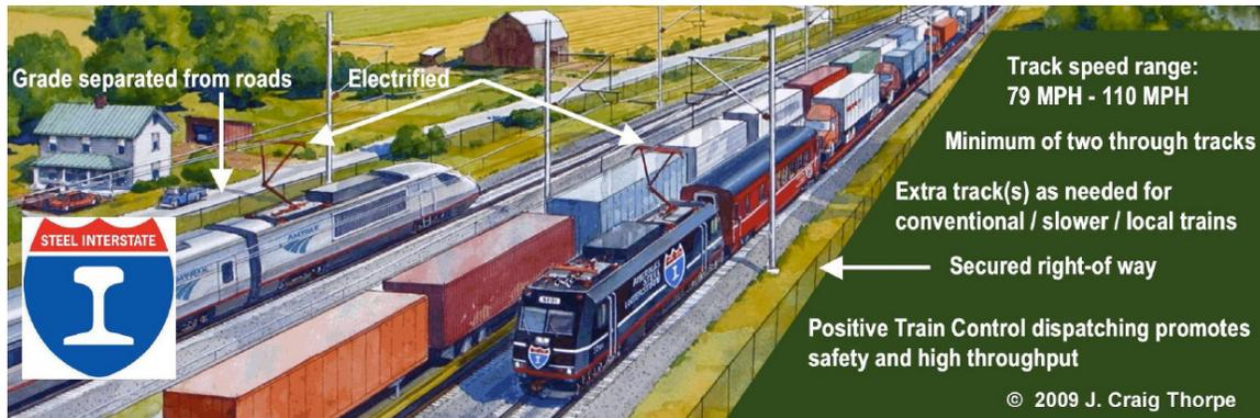
**Figure 1. Features of the Steel Interstate System**
