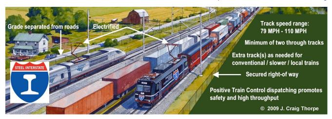
**ELEMENTS OF STEEL INTERSTATE DESIGN:** A minimum of two grade-separated through tracks, engineered, signaled, and dispatched for 79 MPH to 110 MPH, offering frequent, reliable service. The electrified Steel Interstate System would create adequate capacity to divert most non-local truck freight to intermodal trains, and to accommodate passenger trains without impairing freight operations.
