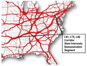
As this FHWA truck density map shows, heavy trucking characterizes this I-81/I-40 Corridor. A similar rail traffic density map reveals only a thin line here. Overwhelmingly the freight flow today is on the highway. Diverting 60% of the through trucks to trains would greatly reduce highway
