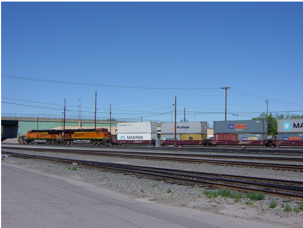
Railroad Double Stack 40' Containers, each roughly equivalent to an “18 wheeler” on the highway
